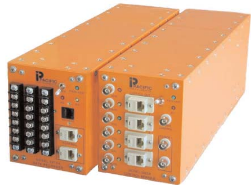
5871-ST - 3-Channel Data Recorder
